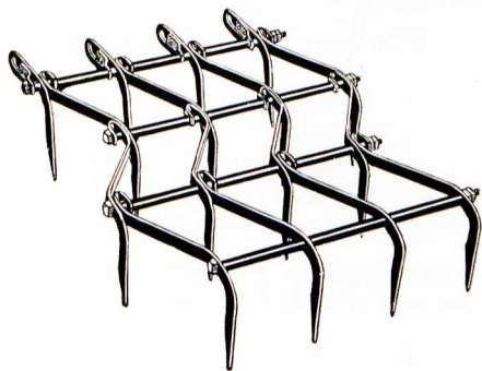
Sunbury Harrows, 16 teeth per section Lines of Cut, 2\frac{1}{4} inches apart
