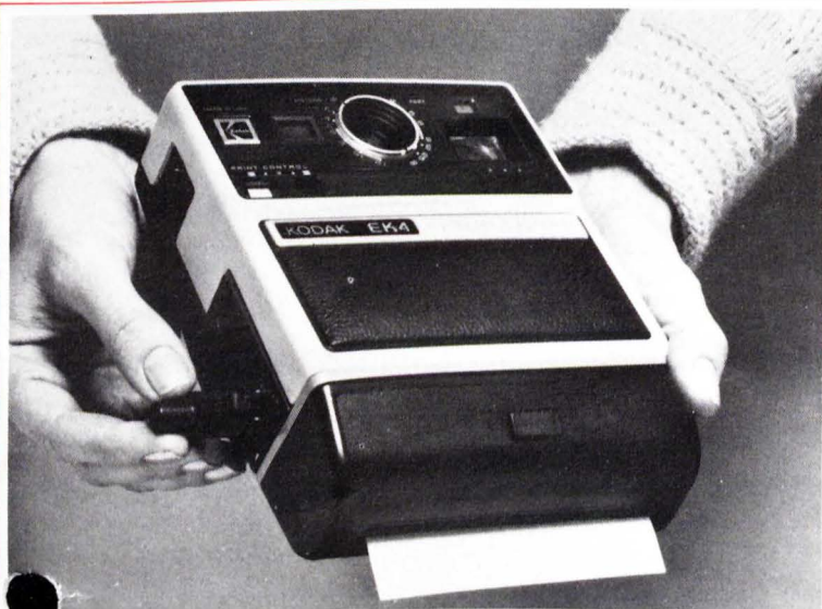
The Kodak EK4 instant camera has an easy-to-use manual film advance which ejects a print from the bottom of the camera after approximately four revolutions of a hand crank. Both the EK4 and EK6 cameras use flipflash.
