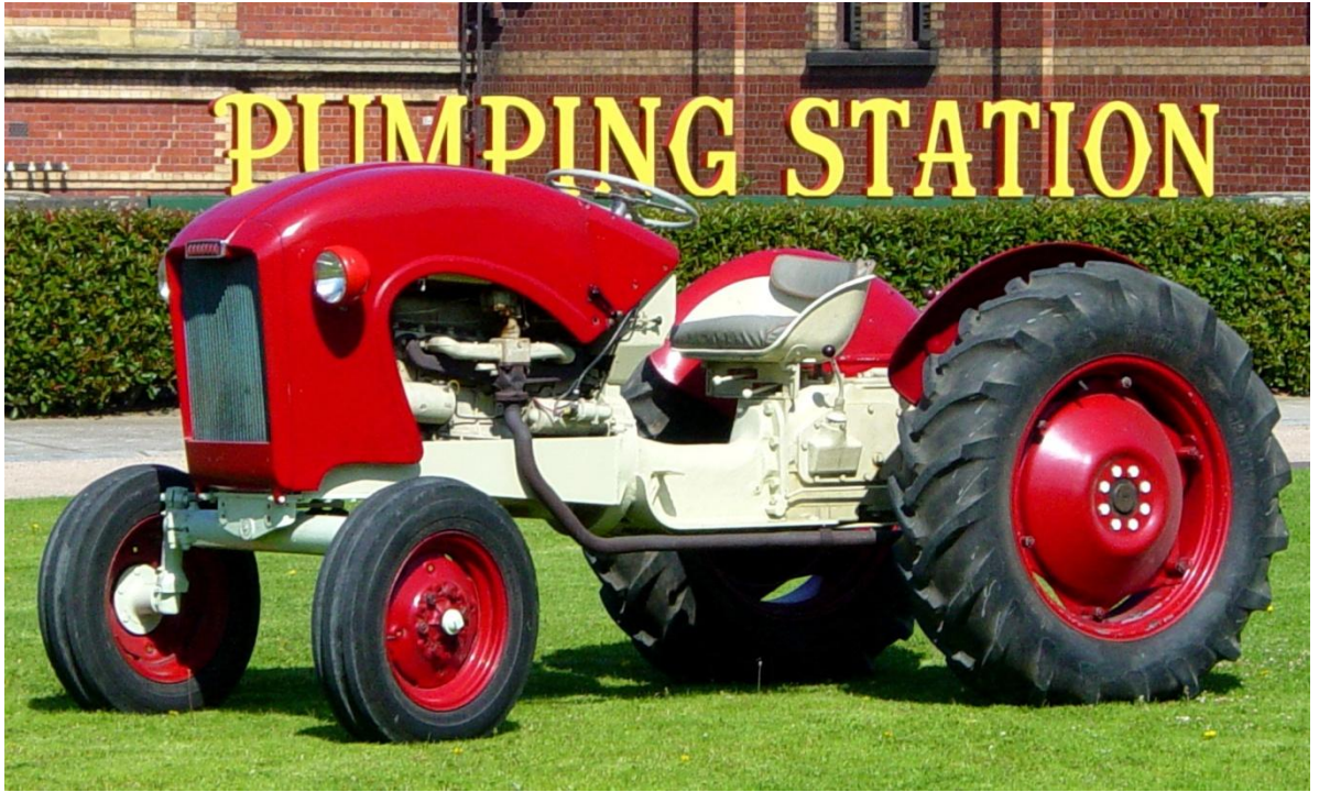
The prototype light tractor produced for Chamberlain Industries in 1959, based on the Holden car engine. This unique Australian-designed tractor now forms part of Museum Victoria's technology collections.
