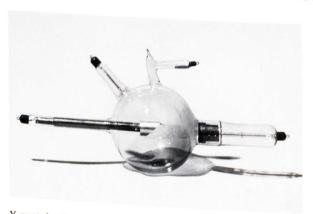
X-ray tubes have undergone many radical changes since Wilhelm Conrad Röntgen discovered x-rays, but the basic principle of producing these rays remains the same. X-rays are generated when fast-moving electrons interact with matter—usually the metal target of an x-ray tube.
