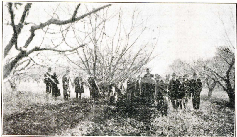
Fig. 5.—Action picture of "Petty" Plow. Note that the Plow is close to the tree whilst the Tractor is driven out clear of the branches.
