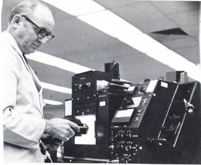
George Bauman reads the integrating instrument as he checks a movie camera into which he has inserted an exposure testing cartridge. Such cartridges are stored, ready for use, in the bin at right. George is in the Customer Equipment Service Center, Kodak Rochester.
