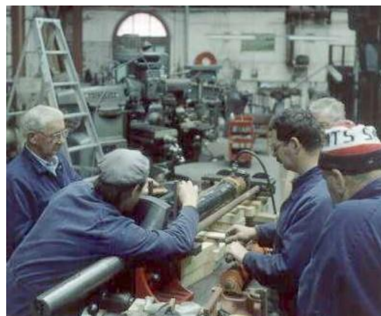
Museum Victoria technical officer, Jeremy Johnstone and volunteers fitting balance weights to the new Cowley traction engine crankshaft, 1997.
