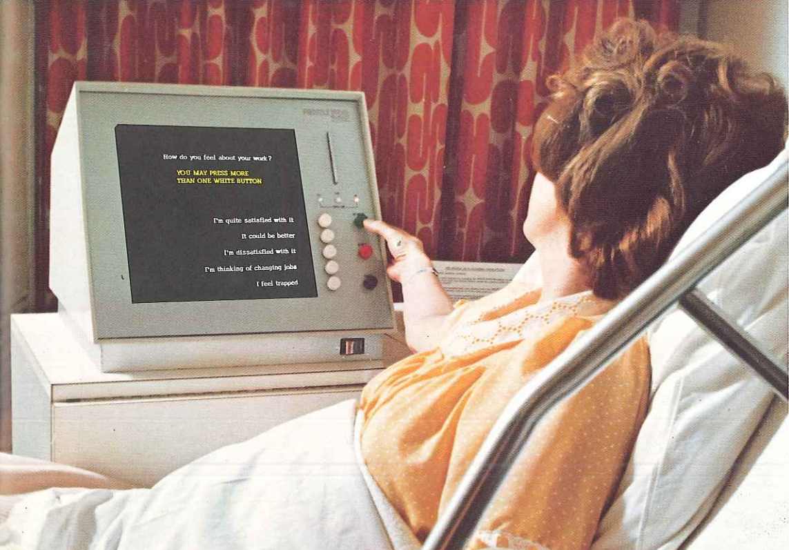
Hospital patient operates Profile 320 History Taker acoustically coupled from her room telephone to a remotely located computer.
