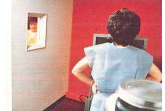
Hospital patient operates Profile 320 History Taker acoustically coupled from her room telephone to a remotely located computer.
