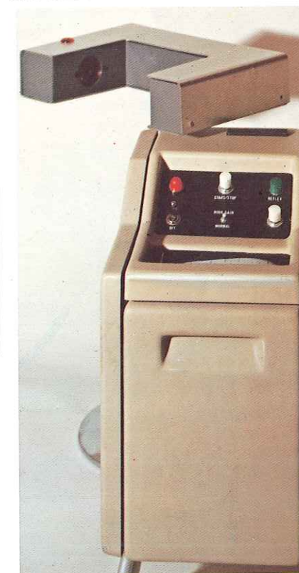
SMI Reflexometer incorporating the Burdick Photomograph Detector and a specialized timing recorder. Inset at left shows the nixie readout
